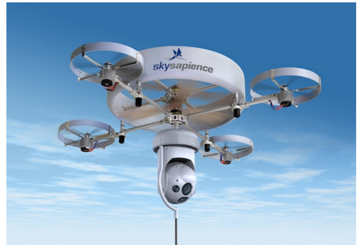
The 'HoverMast' developed by the Israeli start-up company Sky Sapience is an example of hovering camera technologies that are being developed.
